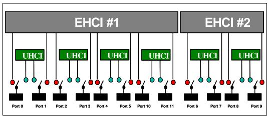
Note that the port-routing logic is the only block of logic within the ICH9 that observes the physical (real) connect/disconnect information. The port status logic inside each of the host controllers observes the electrical connect/disconnect information that is generated by the port-routing logic.
