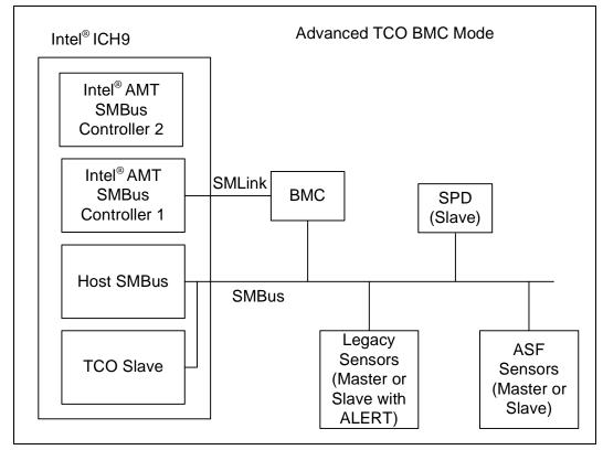
Figure 5-8. Advanced TCO BMC Mode SMBus/SMLink Configuration
