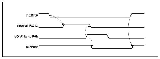
If COPROC\_ERR\_EN is not set, the assertion of FERR# will not generate an internal IRQ13, nor will the write to F0h generate IGNNE#.
