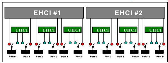
Figure 5-15. Intel® ICH9-USB Port Connections Eight and Four Configuration
