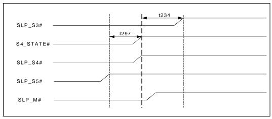
**NOTE:** When both the host and Management Engine boot after G3, SLP\_M# does not have any timing dependency on other sleep control signals. SLP\_M# will be de-asserted some time between SLP\_S5# de-assertion and SLP\_S3# de-assertion.
