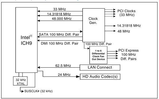
Figure 4-2. Mobile Conceptual Clock Diagram
