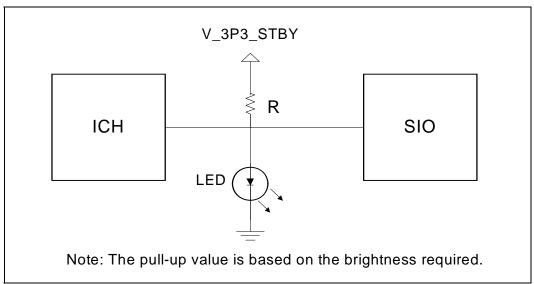
The anticipated usage model is that either the ICH9 or the SIO can drive a pin low to turn off an LED. In the case of the power LED, the SIO would normally leave its corresponding pin in a high-Z state to allow the LED to turn on. In this state, the ICH9 can blink the LED by driving its corresponding pin low and subsequently tri-stating the buffer.
