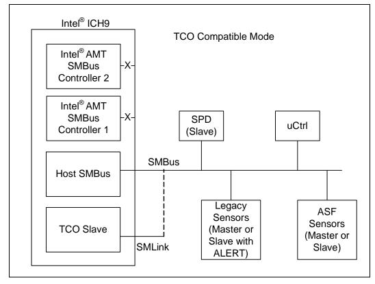
Figure 5-6. TCO Legacy/Compatible Mode SMBus Configuration
